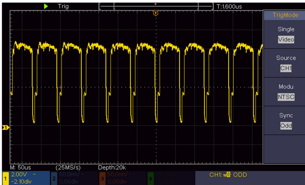
Figure 6-7 Waveform Captured from Video Field Trigger
